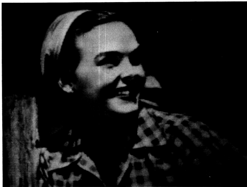
Fig. 7—Reduction of transmission error propagation using predictor output and prediction function leak ( \alpha = 15/16 , \beta = 1/2 , \eta = 128 , 10^{-4} bit error probability).
